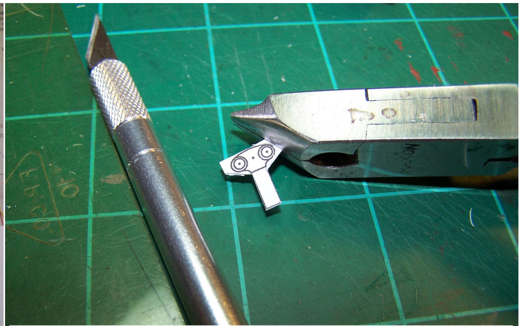
Cut out and sand counterweight to match paper pattern. Remove paper with IPA.
