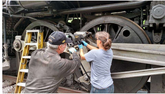
Lube the running gear!
