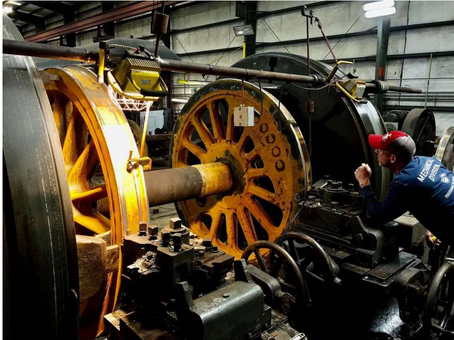
Reshaping driver tire on FMW wheel lathe There sure are a lot of parts!
