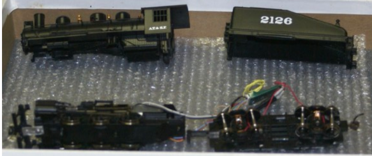
George Van Duyne is reworking a Bachmann 0-6-0, adding wheel pick-ups, TCS decoder, working front coupler and replacing cast on details.
