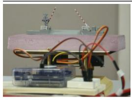
**Terry Cummins** built automated crossings in N Scale using an Arduino and dual servo motors. He also showed a video of the gates in operation on his home layout.
